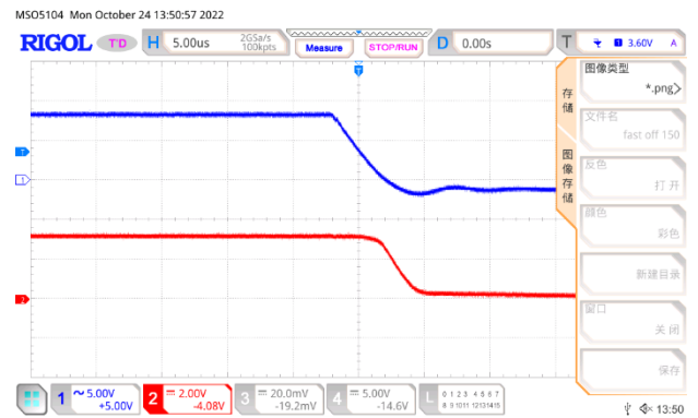
V_{IN} fast off 150mA, V_{OUT}=3.3V
